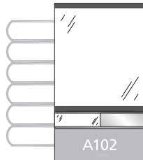
INFOEVWINSL-6L 14-11/16"h x 8-1/2"w (OD) 9-7/16"h x 8-1/2"w Display Insert 10-1/16"h x 8-1/2"w Window (OD) 1-1/2" Slider 3" ADA Insert
